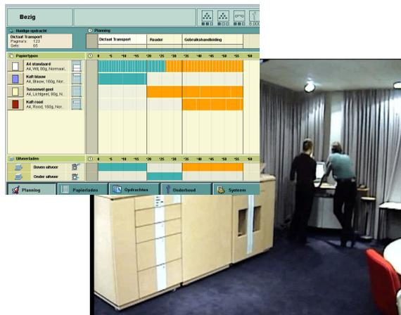
**Picture 2.** The set up of the test performed firstly by Océ employees and later with professional operators. The screen shot (LUI) is the 'Schedule', a tool to be able to plan and program ahead.
