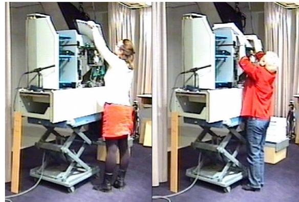
*Picture (1) shows a test where we wanted to learn whether or not users could comfortably reach the upper output tray of a printer. The answer to this anthropometrical question is reasonably objective and we therefore tested with a range of Océ employees.*
