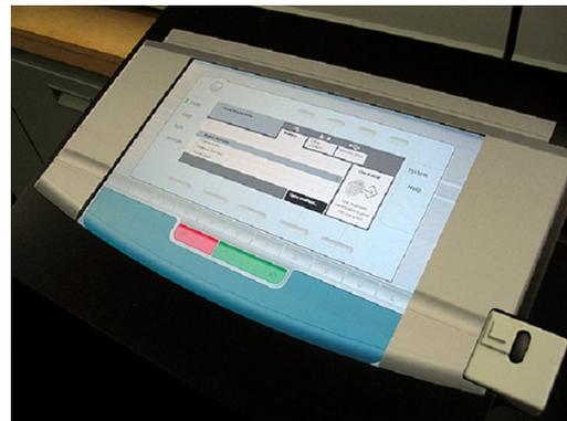
**Picture 5** A prototyped interface, using a touch screen simulating an interface with hard and soft keys.
