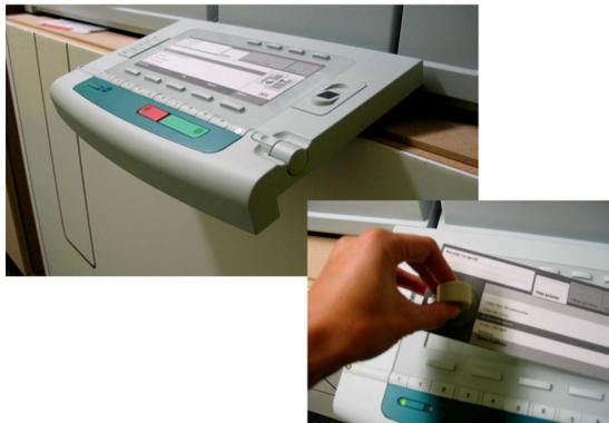
**Picture 4.** Paper prototype in a wooden dummy interface. The 'screens' could be changed easily when a user had chosen something.
